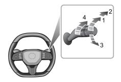
Operate the lever to select different wiping modes:
