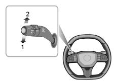
Push the lighting lever downward (1) to turn on the left turn signal lamp; push the lever upward (2) to turn on the right turn signal lamp. The corresponding GREEN indicator lamp in the instrument pack will flash when the turn signal lamps are working.
