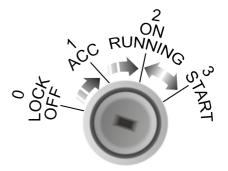
The Key barrel is located on the right side of the steering column. Function of each position is as follows:
