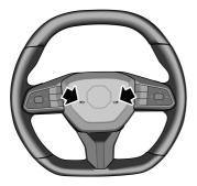
Press the horn button area on the steering wheel (as indicated by the arrow) to operate the horn.
